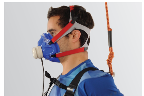
Breath by breath (BxB) mode: Subject wears a multi-use silicone face mask incorporating the flowmeter
