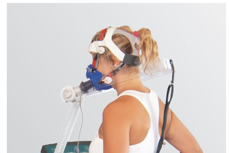
Mixing Chamber (optional) mode: Subject wears a headgear attached to a two-way nonrebreathing valve connected to the mixing chamber
